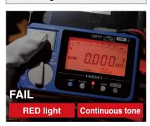
Compare measured values to pre-set reference values to generate a pass or fail decision with the Comparator function.
